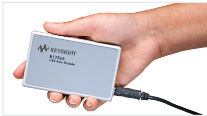
Small and light weight, the Keysight E1735A USB Axis Module allows users to interface the laser, remote control, and optional A Quad B input cable to any PC.
